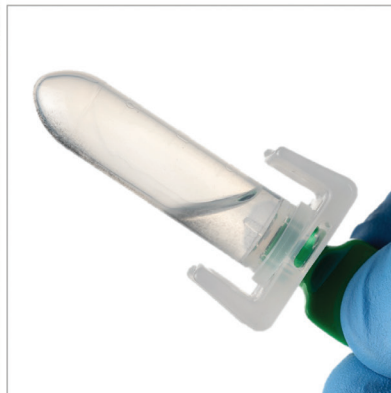
Collect: Inverting the tube with the Magnetic Key collects the magnetic beads onto the SmartLid.
