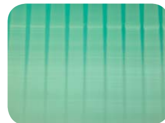
Figure2: High level of detection of protein bands after staining with Reversible Copper stain
