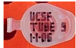
TubeWriter prints on caps of tubes...
